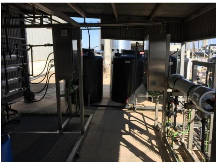
Figure 2.39. Test bed for FO-RO combination research
