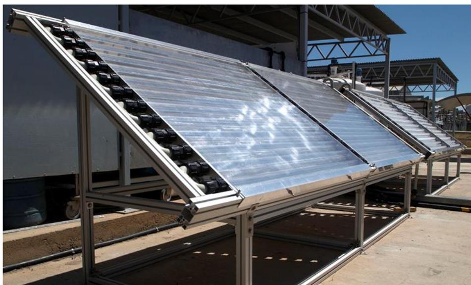
Figure 2.40. CPC photo-reactors (SOLEX prototype).
