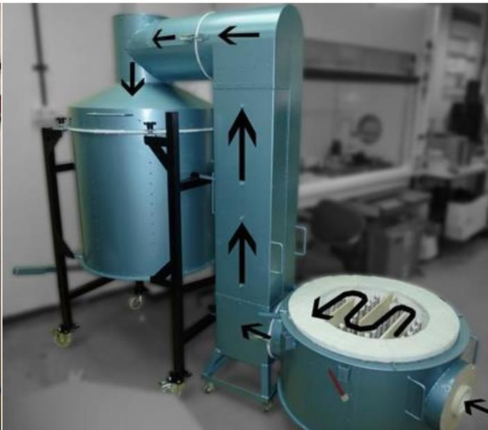
Figure 2.30 Front view of the lab-scale regenerative storage system in dynamic arrangement.
