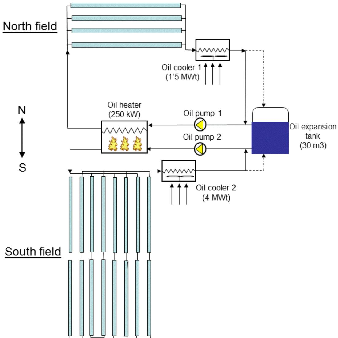
Figure 2.11. Simplified scheme of the PTTL facility
